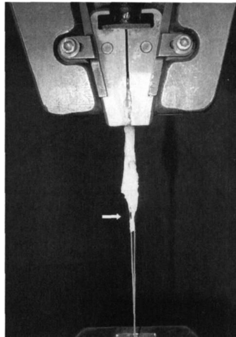
**Fig. 6:** All specimens failed by pulling the suture material out of the tendon.
